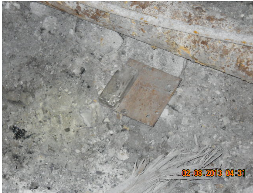
Safety Switch Actuator on the Ground During Accident Investigation
